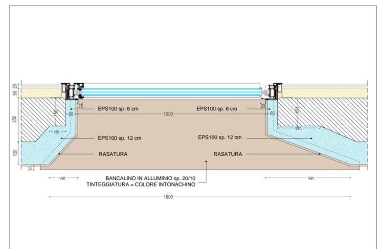
DETTAGLIO SPALLETTE FINESTRA 100x100 cm PROSPETTO OVEST
