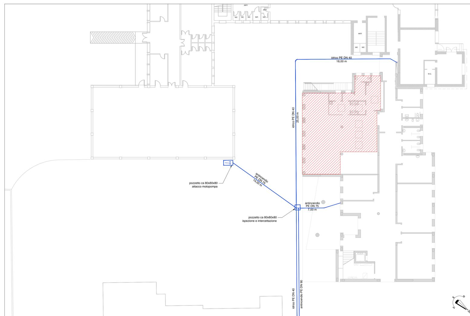
PLANIMETRIA DI DETTAGLIO CON EVIDENZIATA LA RETE IDRICA E RETE ANTINCENDIO DI PROGETTO
